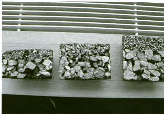
Figure 1. Examples of two-layer drainage asphalt. From left to right: DA5 + DA16, DA8 + DA16, and DA5 + DA22.
