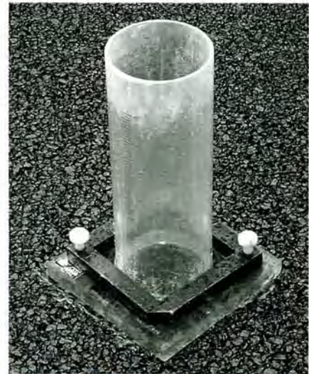
Figure 12. Permeability testing of recycled mix.
