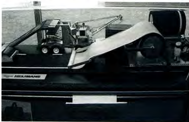
Figure 9. Construction of the rollable road.
