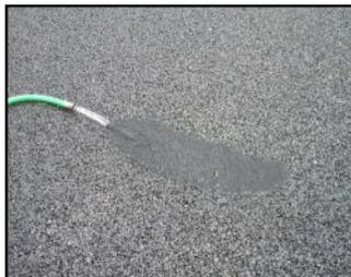
In an effort to promote “greener” pavement structures and materials, VAA and VDOT have been working on developing specifications and guidelines for porous asphalt pavement structures.
