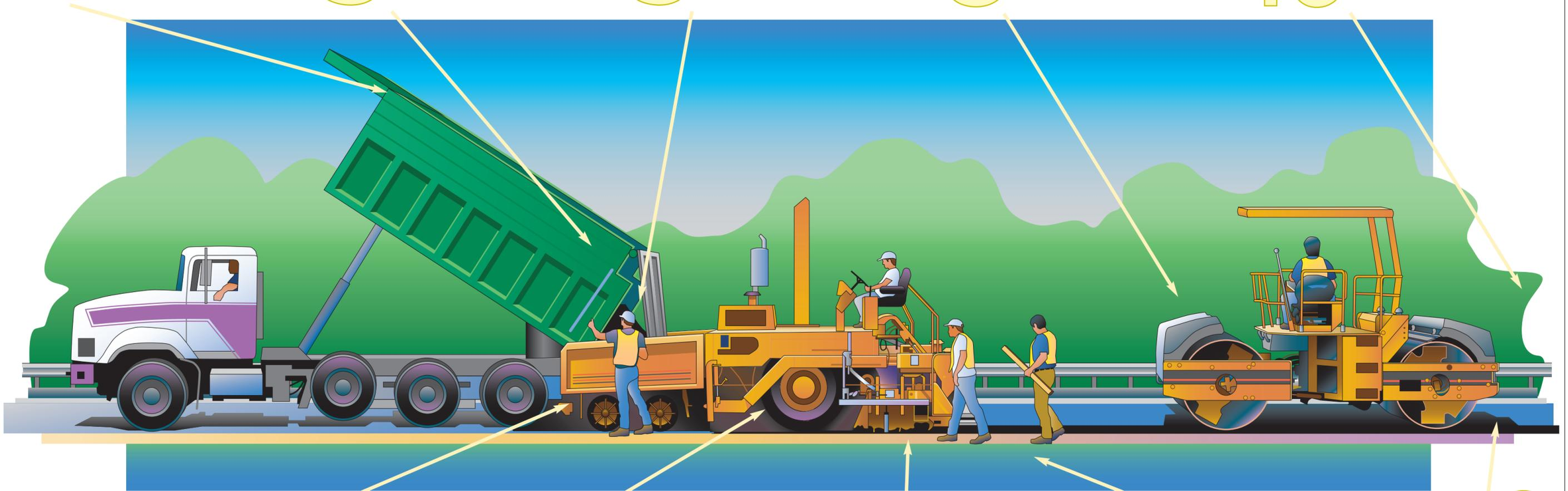
2. The truck driver backs up just short of the paver – the driver should be careful not to bump the paver. Once the paver makes contact with the truck, the driver raises the bed. The truck driver applies the brakes gently, and the tractor unit on the paver pushes the truck forward.
